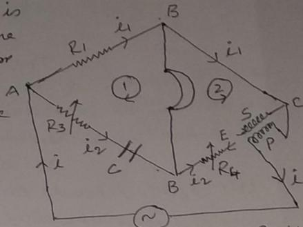
variable non-inductive resistance  $R_3$ . The other coil P of the mutual inductor is connected in series with the source. The balance condition is not given by usual general condition of an a.c bridge. Let 'i' be the instantaneous current in the source branch,  $i_1$  through  $R_1$  and  $i_2$  in ADC branch at balance of the bridge.
